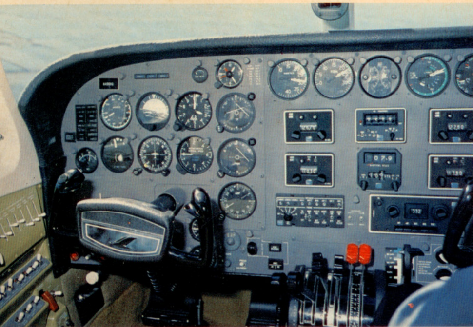
Electronic checklist is at far upper-left-hand corner of main panel on the Cessna 340; cabin pressurization control is at bottom of panel, to right of control wheel. Taken in flight, photograph shows the 340 cruising at 3,000 feet, using 29 inches manifold pressure and 2,300 rpm. Radio equipment is Cessna 400 series (made by ARC) and DME is King. That's a digital ADF at bottom right of panel.
